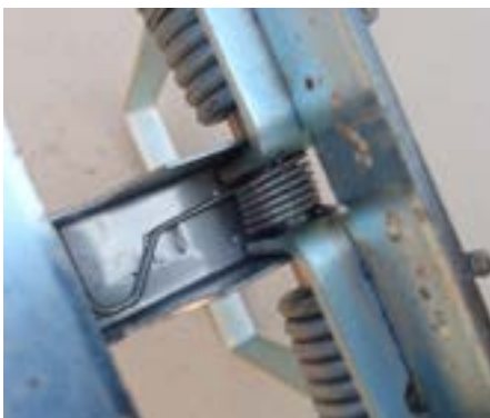
The configuration of the DOC trap with multiple strike bars, a strategically placed baffle and plenty of power significantly increases the likelihood of a humane dispatch.
