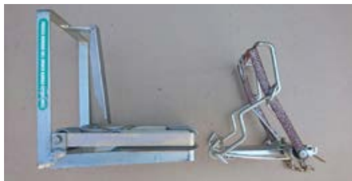
DOC traps are marginally taller than their Fenn-type equivalents so existing tunnels may need adapting. This photo shows the difference in height between a DOC 200 and a closed Fenn-type Mk 6.
