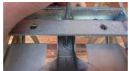
The sensitivity of the treadle plate can be altered by adjusting the sear nub by gently tapping it either from above or below using a light hammer and punch (in this case a steel tent peg).
