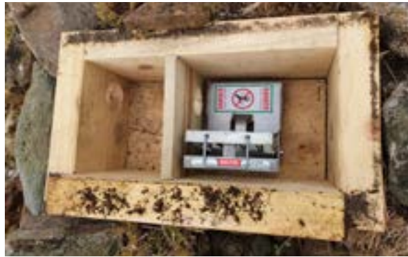
Correct DOC trap position for a single-entry tunnel – note the gaps between treadle plate and box side and between trap and inner baffle are both within the legal 10mm limit. Because this is a single-entry tunnel, the larger gap to the right of the trap is not likely to cause an inhumane catch, and can be used to add a bait if desired.
