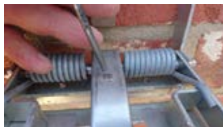
The sensitivity of the treadle plate can be altered by adjusting the sear nub by gently tapping it either from above or below using a light hammer and punch (in this case a steel tent peg).
