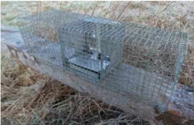
DOC 150 traps lend themselves to being used on rails, but it is imperative that every effort is made to exclude non-targets, as well as ensuring the correct gaps between treadle plate and tunnel side and between trap and inner baffle are maintained at no more than 10mm.
