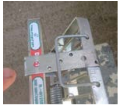
We advocate the use of folded metal fixing strap to hold open the jaws of traps when working on them.
