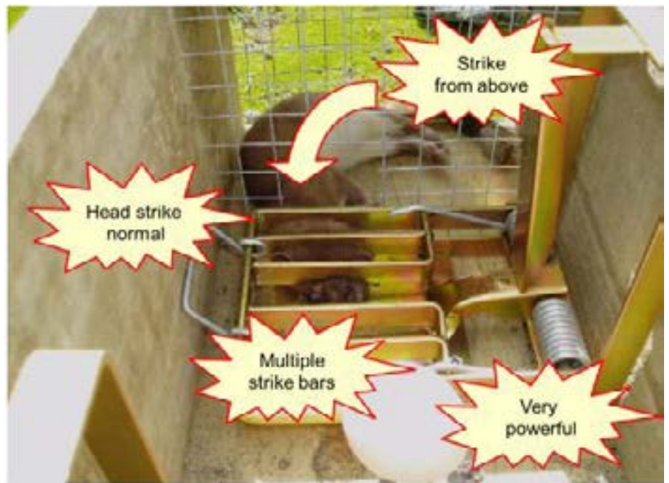
The configuration of the DOC trap with multiple strike bars, a strategically placed baffle and plenty of power significantly increases the likelihood of a humane dispatch.
