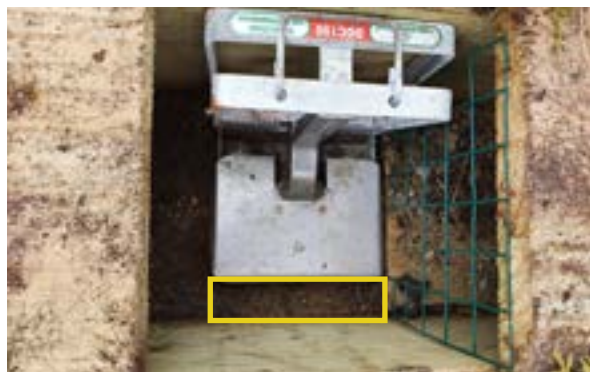
Incorrect DOC trap position – note the gap (highlighted in yellow) between treadle plate and side of box is in excess of the legal maximum of 10mm.
