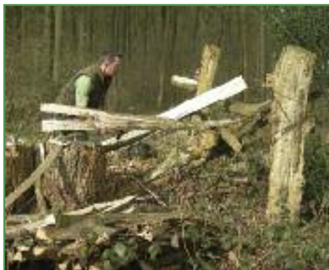
Phil Winterton making riven rails from ash poles in Tugby Wood.
