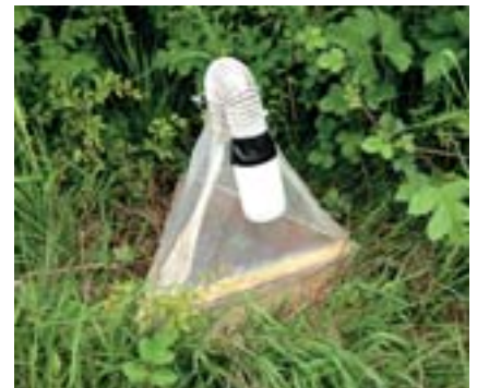
Emergence trap used to assess use of non-crop habitats by invertebrate predators of crop pests.
