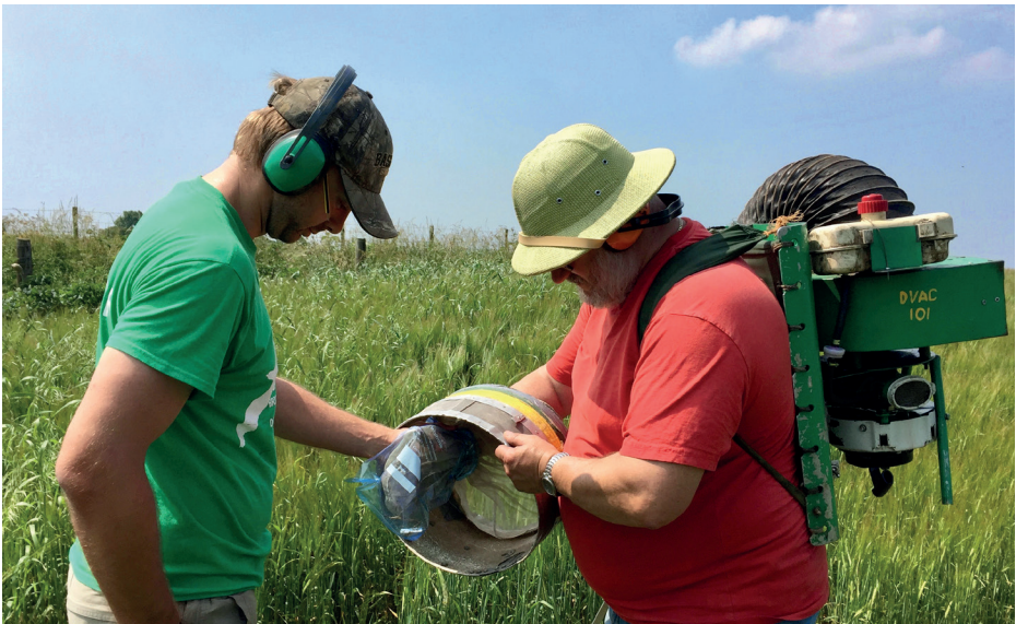
We still use a traditional DVAC to collect samples in order to ensure consistency.
