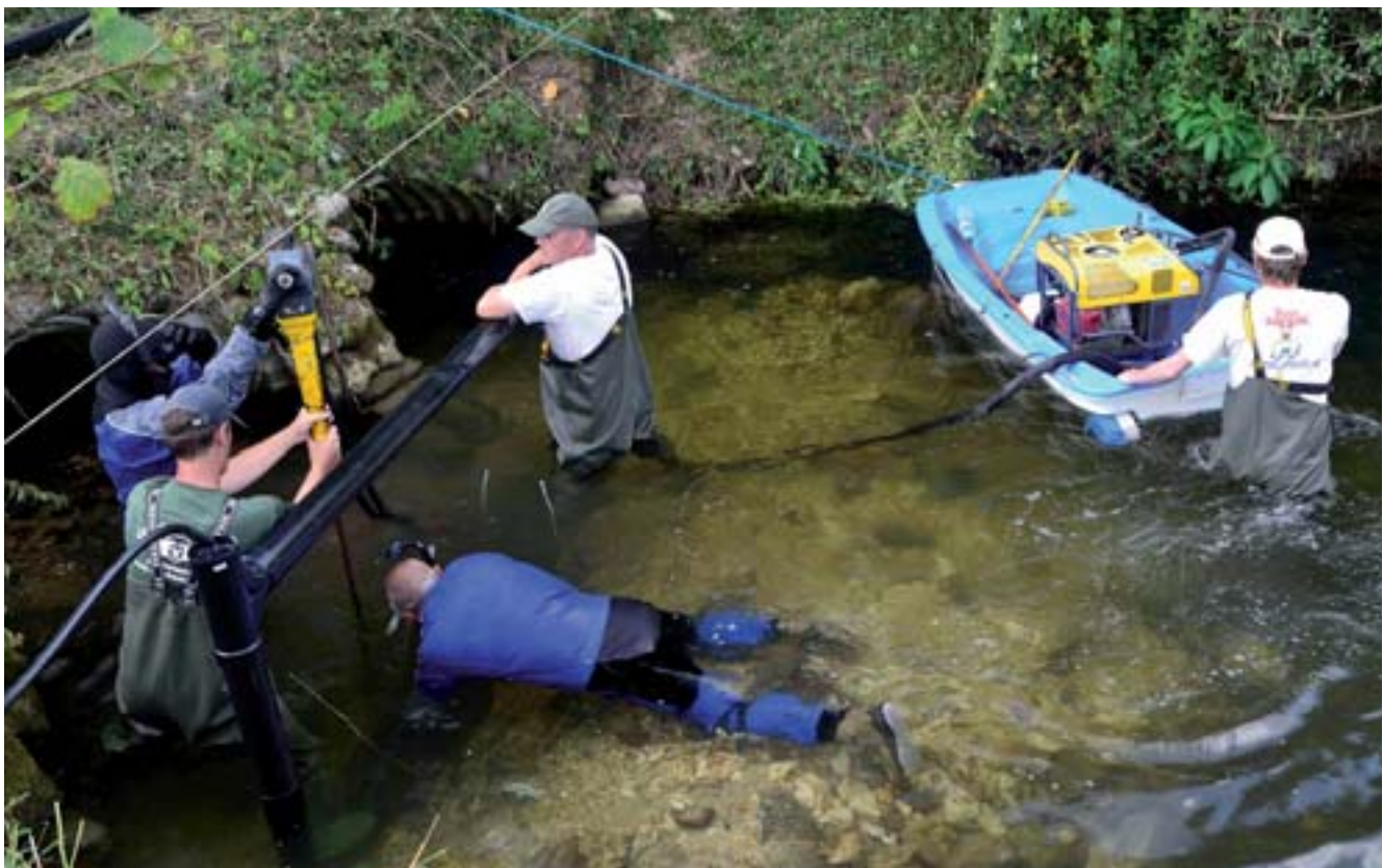
Installing new antennae that will count the number of salmon on the River Frome. © Dylan Roberts/GWCT
