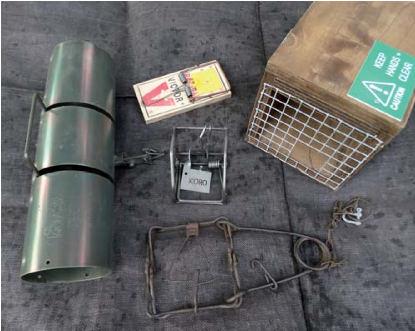
It isn't clear yet which traps will be approved for stoats after testing is complete. New traps may emerge, but initially there was only a short list of possible contenders. Clockwise from left: WCS Tube Trap, Victor EasySet Rat Trap, DOC trap (in tunnel), BMI Magnum 116, and (centre) Koro Small Rodent Trap. © Mike Short/GWCT
