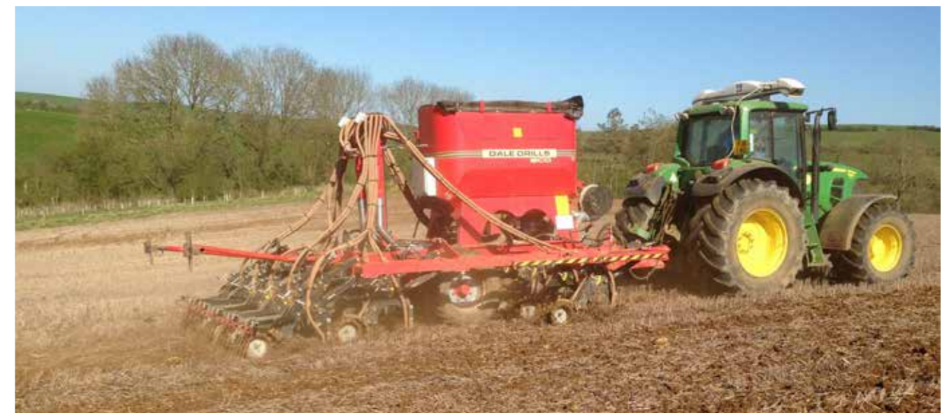
Figure 18: A Dale seed drill purchased by the Welland Valley Partnership to encourage farmers to adopt direct drilling in the study area.
