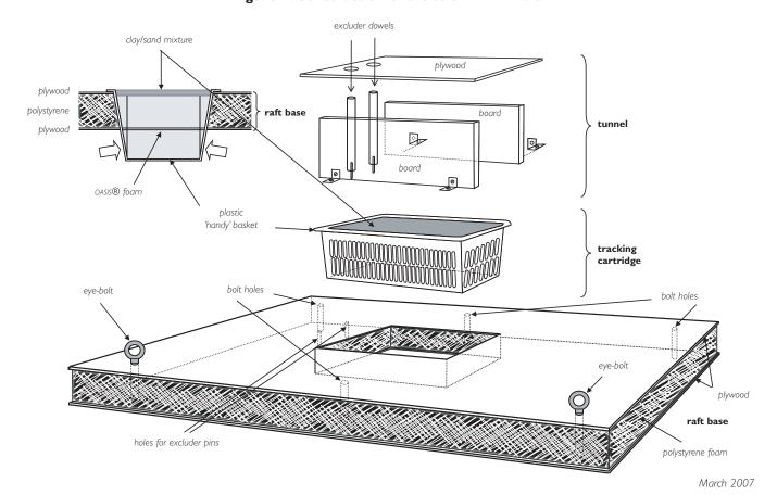
Figure I. Construction of a GWCT Mink Raft
