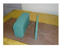
**Step 2:** Cut the two wedge-shaped pieces, referred to in the diagram as parts B and E. The thick end of the wedges should be 20mm deep. Both cuts should be made from the corners of the same side and angled inwards, so that the main block becomes shaped like the basket. It is useful to score cut-lines before removing the wedges. In the diagram the main block is referred to as part A.
