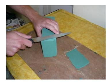
**Step 3:** Take the thin layer that you removed in Step 1. Cut it lengthways, to give you two strips, one 65mm wide (part C) and one 45cm wide (part D). Cut two wedge-shaped pieces from either end of part C. The thick end of the wedges should be 20mm deep. As before, both cuts should be made from the corners of the same side and angled inwards.
