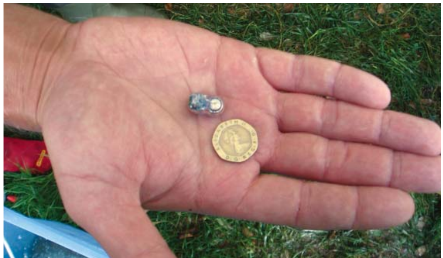
A radio-transmitter used in our radio-tracking experiment with a 20p piece for size comparison. (Brian Shields)
