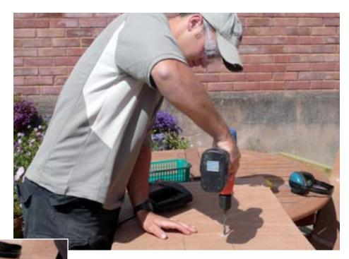
(Above) Drill a pilot hole to insert the jigsaw blade. (Left) Use your jigsaw to cut a window in your sheets of plywood.
